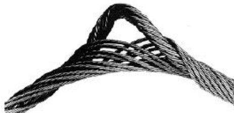
Figure 10, Core Protrusion, Indicating Shock Loading
